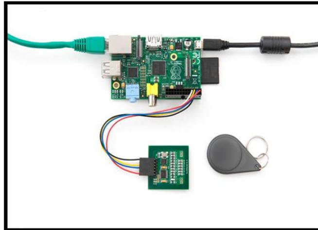
**Fig. 2** RFID and Raspberry Pi Interface
